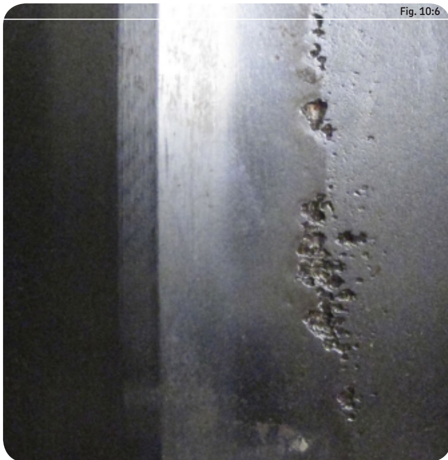
Spalls and surface distress on the raceway of the same felt roll bearing taken at f2.8 1/100s and ISO 3200
