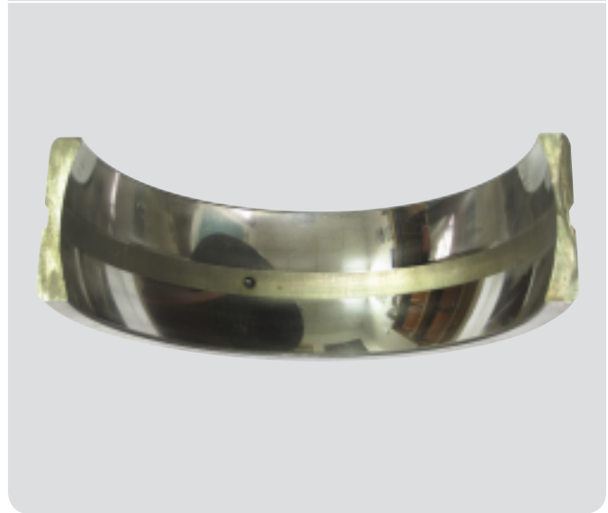
Polishing wear on the outer ring of a spherical roller bearing mounted on a felt roll in the dryer section
