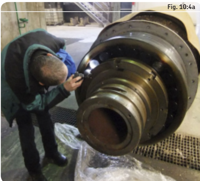
Fig. 10.4a and fig. 10.4b: A press roll bearing mounted on a journal is cut in a place without visible damage
