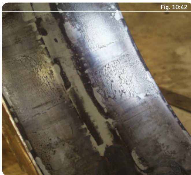
Suction press roll bearing with too much water in the lubricant
