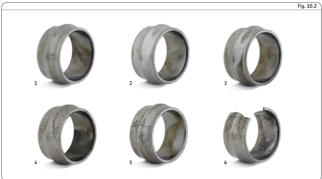
The development of bearing damage
