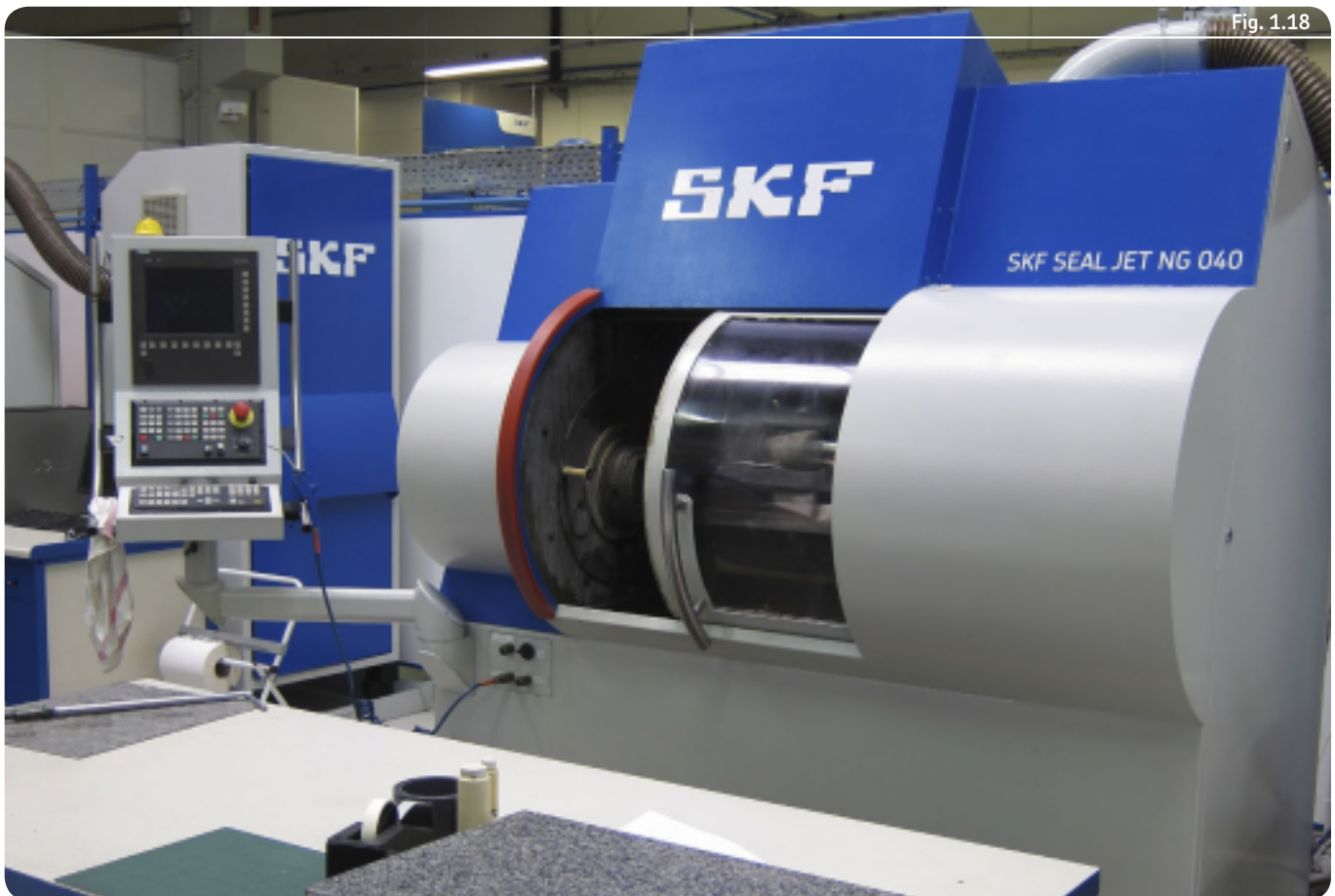
SKF Seal Jet: CNC machine to manufacture customized seals
