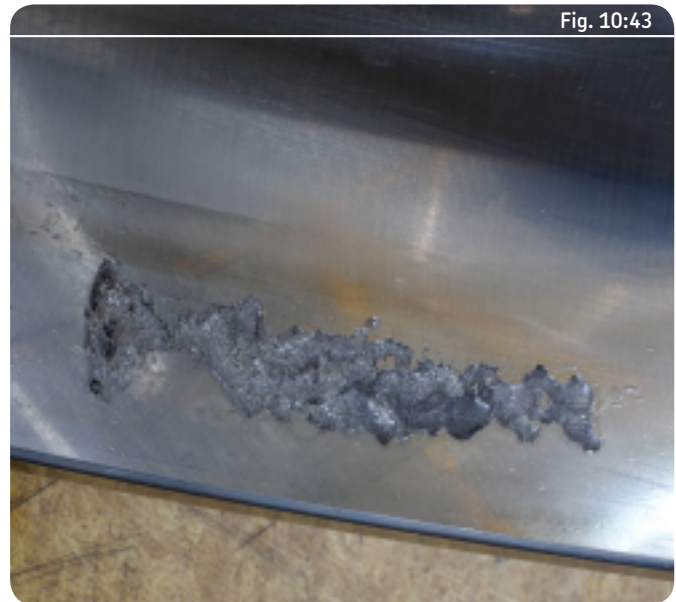
Spalling created by a single instance of deep-seated contact corrosion on a drying cylinder bearing. The spall has propagated first in the axial direction at the initial damage and then has propagated in the rolling direction (left to right).
