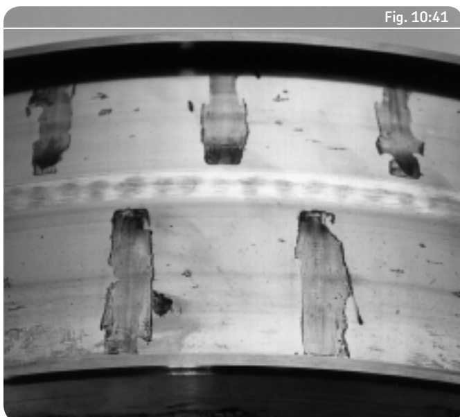
Standstill corrosion under static conditions
